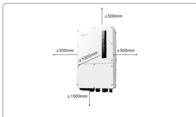
Fig. 4-17 Inverter Mounting Clearance
